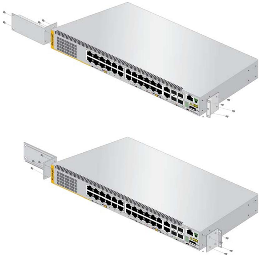
Figure 19. Installing Brackets on the AT-x310-26FT Switch
